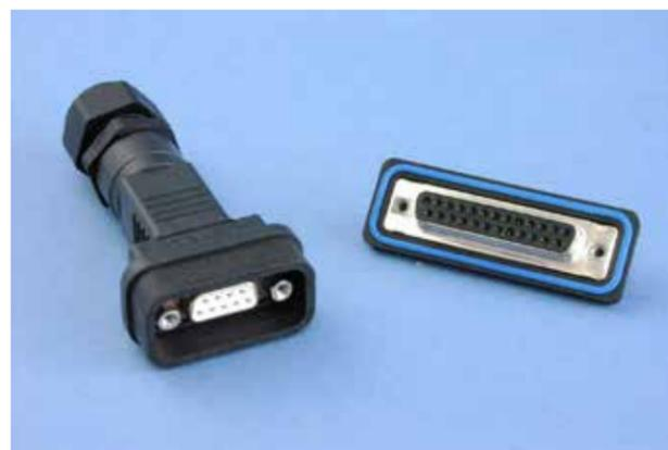
In2Connect now offers Nano 'D' subminiature connectors with an 0.025" pitch: plugs and sockets, in 9, 15, 21, 25, 31, 37, 51 and 69 ways for termination on printed circuit boards or attached to cable assemblies. Ideal for mission critical applications like aerospace, aviation, electronic, and military communications, these connectors are militarily unique because of requirements to operate satisfactorily under sinusoidal vibrations of 10 to 2000 Hz at up to 20 g's.
